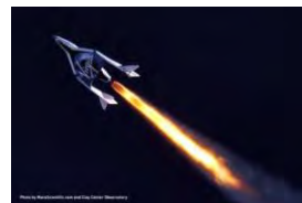
Nitrous Oxide (N 2 O) Oxidizer HTPB or Polyamide Based Fuel
