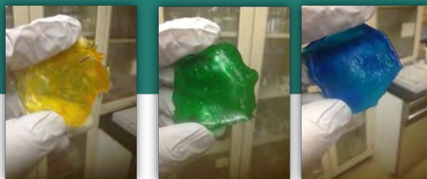
Bioplastic films made from corn (yellow), potato (green), and tapioca (blue) starch
