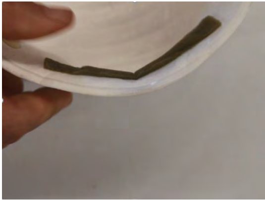
Nosefoam after 1 cycle loses ability to recover to full thickness, which compromises fit performance.
