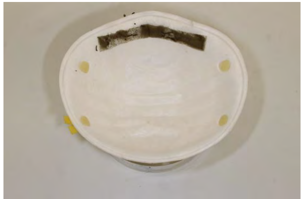
After multiple cycles, nosefoam degrades completely.
