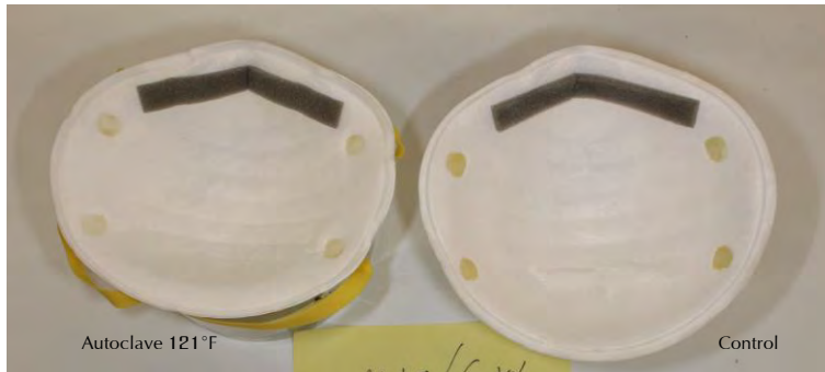
At high temperatures, the respirator shrinks considerably, which compromises fit.
