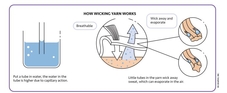
clothing is polyester. Being petroleum based, polyester is quite hydrophobic, with a moisture regain of only 0.4%. To make it a little less so, it can be chemically treated with a hydrophilic coating. Or the polyester fibers may be interwoven with hydrophilic fibers, forming a blend, which can create an excellent moisture-wicking garment.
