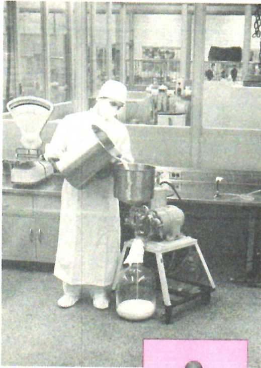
In Sterile area, George Kramer runs suspension through colloid mill to disperse particles.
