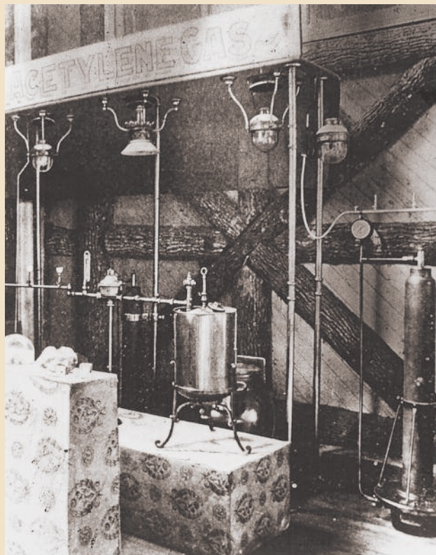
Acetylene generator, compressed gas cylinder, and acetylene lights, on exhibit at the Atlanta Exposition, August 1895.
