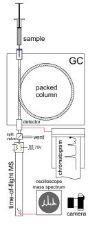
This schematic shows the major components of an early gas chromatographmass spectrometer. Not to scale. Credit: Mark Jones
