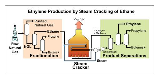
Raw natural gas is purified to remove impurities and natural gas liquids (NGL). The natural gas liquids are then fractionated to give pure ethane, propane and higher molecular weight components. Ethane is converted to ethylene and hydrogen upon heating in a steam cracker. Credit: Mark Jones
