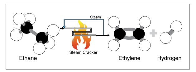
In a steam cracker, ethane is converted to ethylene and hydrogen by brief heating in an empty tube with steam, which is added as a diluent. The hydrogen is burned to provide heat for the reaction and subsequent processing. Credit: Mark Jones
