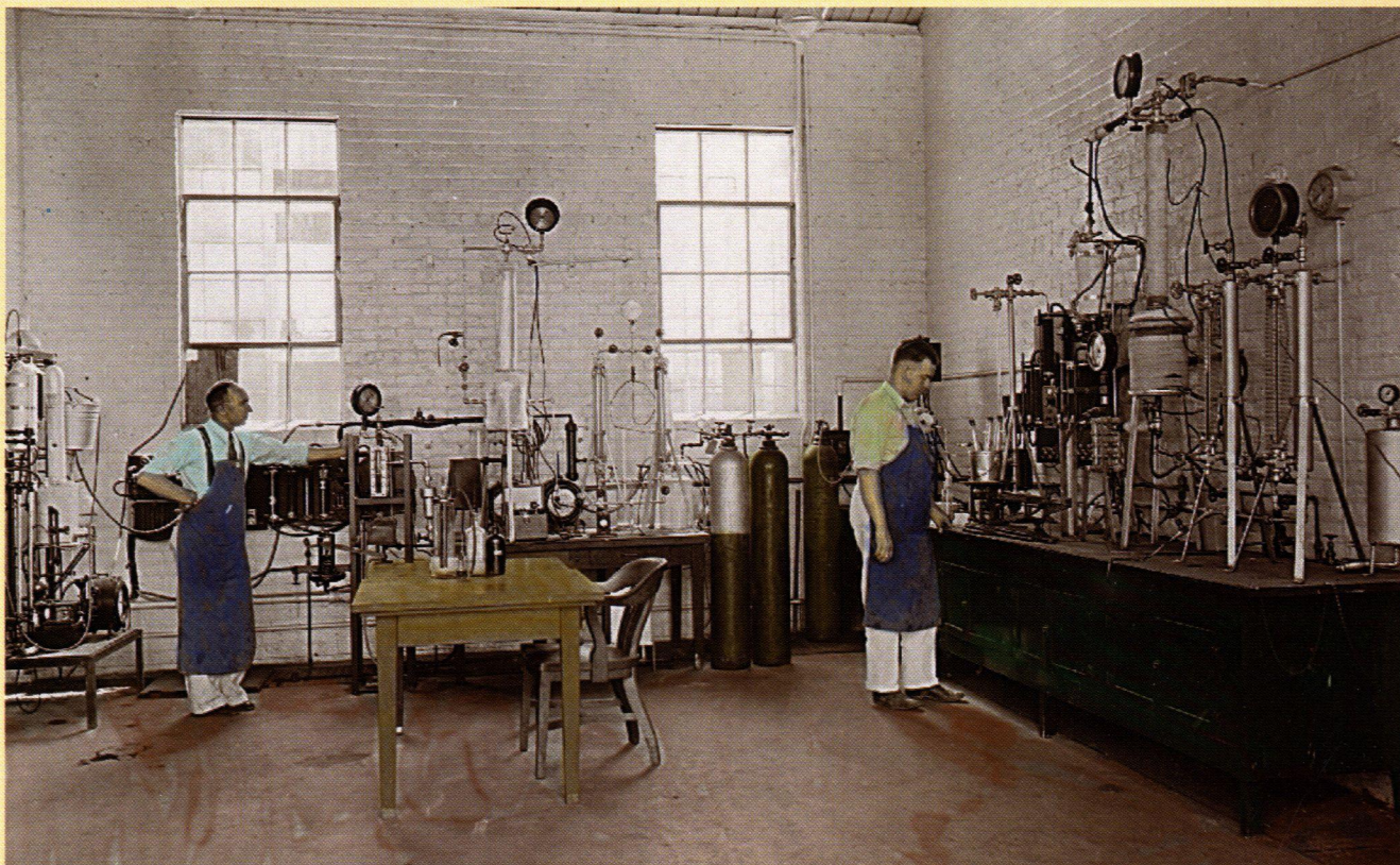
A laboratory pilot plant at Riverside. The lab, circa 1920, was used for studying the Dubbs process.
