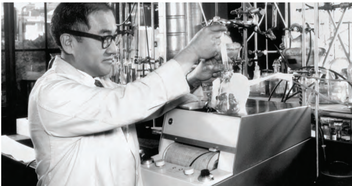
Roy Teranishi samples the headspace over fresh grapes before injecting a sample into a gas chromatograph.
