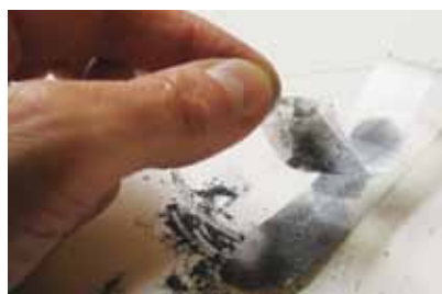
Sticky tape can be used to peel off powdered graphite, leaving a single layer of graphene.
