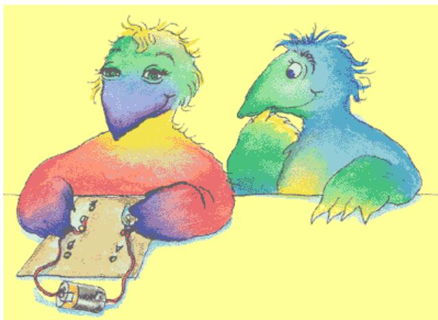
7. Touch the bottom of the bulb to one brass fastener and the end of the wire to another. If the hidden wire is connecting those two fasteners, the circuit will be complete, the bulb will light, and you will have found the hidden wire.
