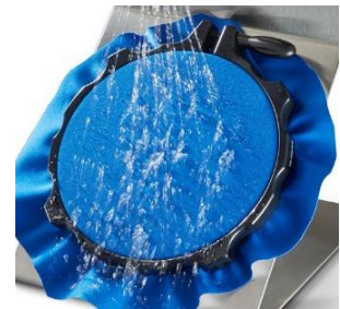
Spray test BS EN ISO 4920 Industry standard for testing resistance to surface wetting
