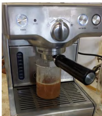
Figure S1: Extraction of star anise using an espresso machine.
