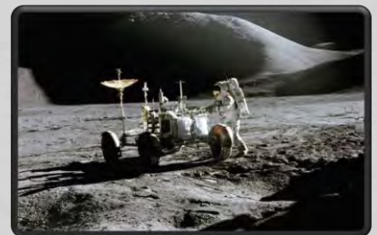
Apollo 15-Astronaut James B. Irwin, lunar module pilot, works on the Lunar Roving Vehicle
