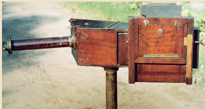
Although Raman’s original experiments were done by visual observation, precise measurements were made with this quartz spectrograph and first made public by Raman in a lecture in Bangalore on March 16, 1928.
