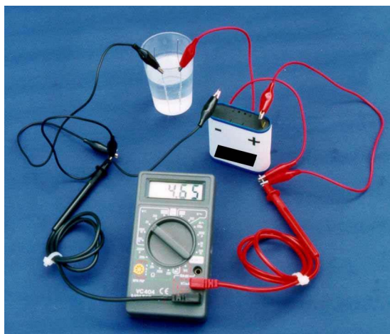
Figure 3: Photo of Electrolysis Experiment Set Up Source: Courtesy of Dr. Martin Schmidt, "Platinum Fuel Cell Kit Instructions" http://www.geocities.com/fuelcellkit/pdf/FC1101e.pdf
