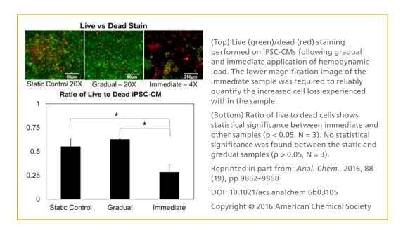
To simulate the conditions of damaged heart tissue, the researchers flushed the culture chamber with serum containing few nutrients, and noticed that many cells died.
