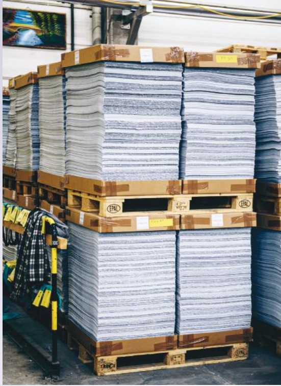
Renewcell dries pulp made from waste cotton into sheets that are then sent to fiber producers.
