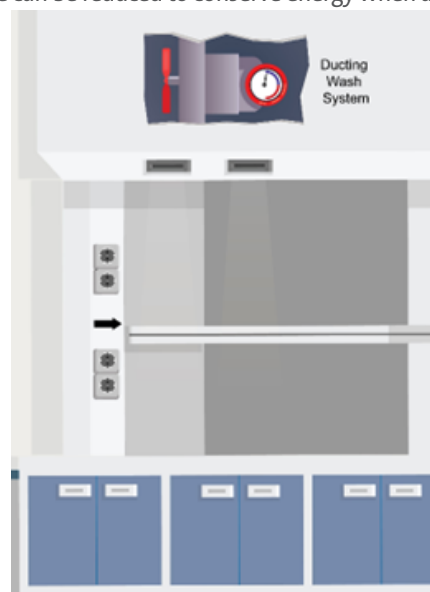
Figure 3: Perchloric acid hood with washdown system for the hood and duct.
