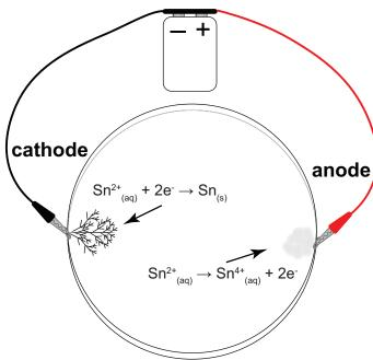
**Electrolysis of tin(II) chloride.** Tin(II) chloride is reduced at the cathode to tin metal crystals. At the anode, it is oxidized to  $Sn^{4+}$ , which reacts with chloride ions present in the solution to precipitate out as tin(IV) chloride.
