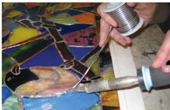
Figure 4. Molten solder flows onto the seams and creates a "came."
