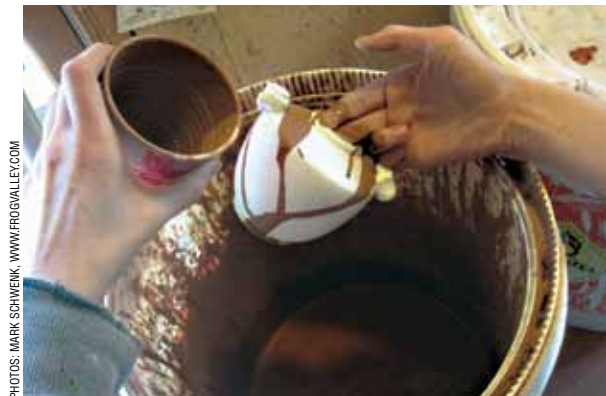
Above: Glazes rich in metallic oxides and carbonates are applied to a pot before it is fired in a kiln.
