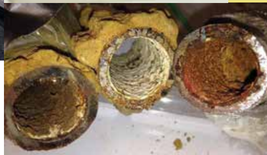
Above left, Otto Schwake, a postdoctoral microbiologist at Virginia Tech, tested Flint tap water for waterborne pathogens. Top, water flowing from a faucet in a hospital in Flint, Mich. Above, pipes from the Flint water distribution system after the city decided to use water from the local Flint River.
