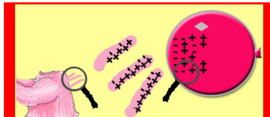
The positively charged fibers are now attracted to the negatively charged balloon.
