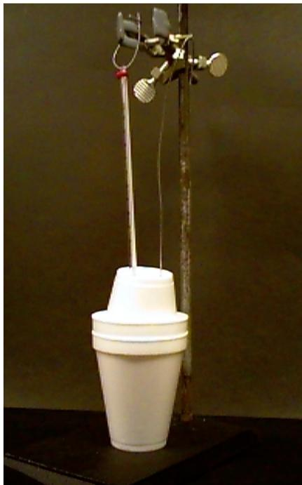
*Notes:* The inner cup can be replaced as needed, which is why there are extra foam cups. 250 mL (8 oz) foam cups may also be used but 190 mL (6 oz) cups are not recommended. You may choose to supply a ring clamp to stabilize the base of the cup assembly. Another option is to place the cup assembly in an appropriately sized beaker that serves to support the cups and to provide extra insulation.
