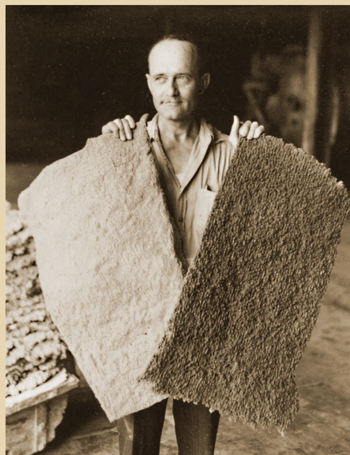
Sheets of dried synthetic rubber (left) and dried natural rubber (right).
