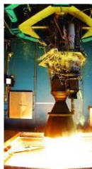
Merlin 1C 147 to 161 klb Thrust
