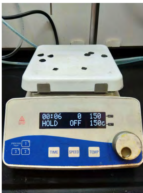
Figure S1. The electrodes can be dried overnight. Make sure to note which electrodes are the anodes and which are the cathodes.
