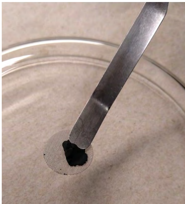
Figure S3. Spreading the anode slurry onto the stainless steel mesh current collector.
