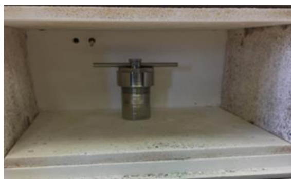
Figure x: PTFE-lined stainless-steel autoclave setup used for the hydrothermal synthesis
