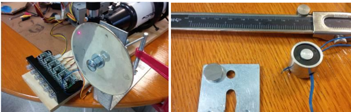
Figure 3 (r): A mirror sample is firmly mounted in a test stand by the center hole. (l): Two different magnetic actuators have been tested: A solenoid that at 12v produces 25N force against an iron plate (upper right). And a stack of two N48 Neodymium rare earth magnets 2mmx13mm each (seen in the lower left attached to the metal plate).
