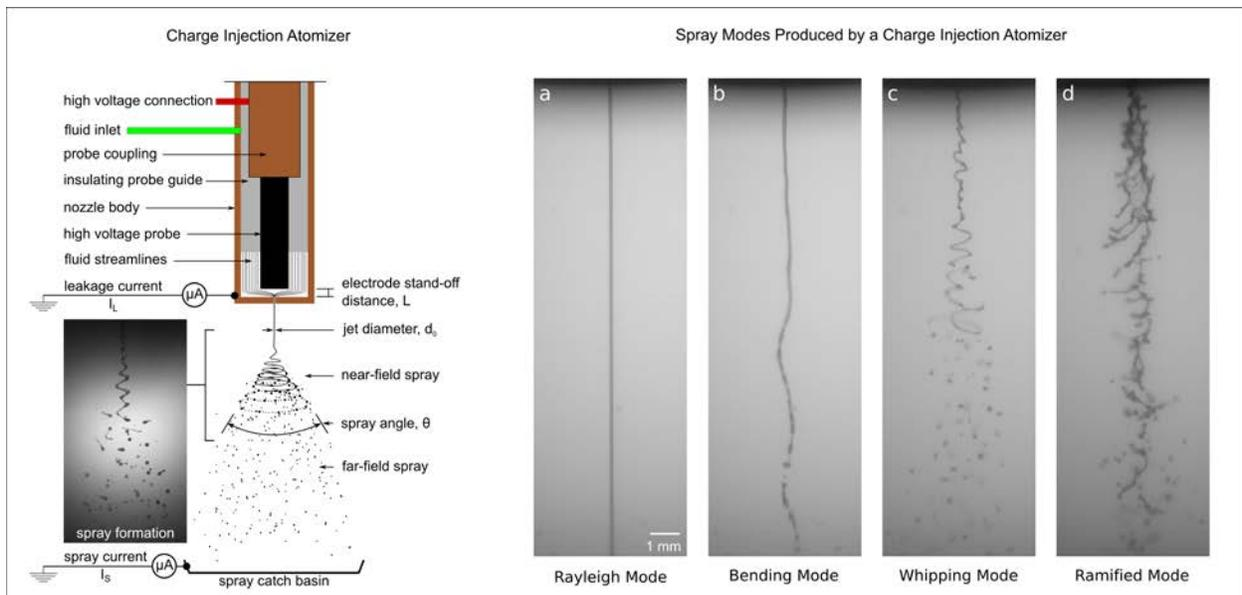
**Graphical Abstract:** (left) Schematic of setup used for the electrohydrodynamic atomization of dielectric fluids. (right) Spray mode progression for increasing applied potential.
