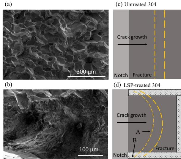
**Fig. 2.** (a)-(b) SEM images of fracture surface of LSP-treated 304 steel: (a) in the center (indicated by A in d); (b) near the surface of the specimen (indicated by B in d). (c)-(d) Schematic diagram of crack growth process in the cross-section of (c) untreated 304 steel and (d) LSP-treated 304 steel.
