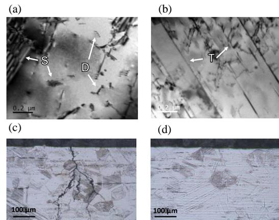
**Fig. 1.** (a)-(b) TEM images of near-surface microstructures of ODS 304 steels after LSP. S: stacking fault; D: dislocation; T: deformation twin. (c)-(d) Optical micrograph of the cross-section microstructures after SCC test of 72 hours: c) untreated 304 steels; d) LSP-treated 304 steels.
