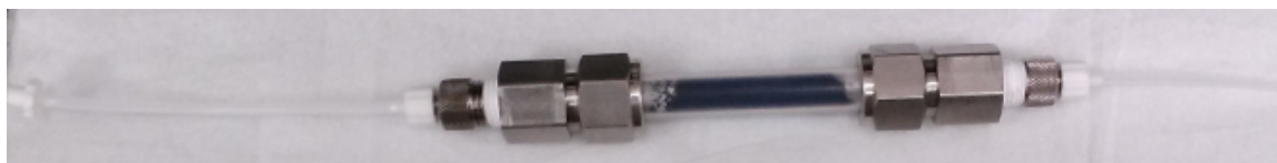
Figure 1. Column apparatus for assessing dispersant adsorption onto carbon black.
