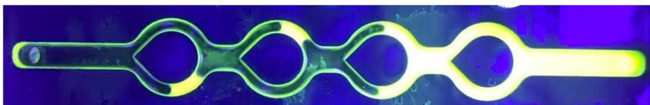
**Figure 1.** a) Top view of aqueous solution in process of displacing dyed silicone oil 20 cst. Flow is from left to right.
