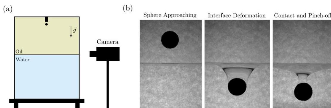
**Figure 2.** Motion of a sphere through an oil-water interface. a) Sketch of the experimental apparatus. b) Steps during the falling of a *rough* sphere through the interface captured by a high-speed camera.
