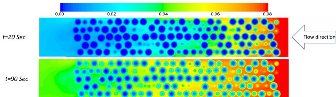
Figure 2.  $O_2$  mass fraction profile along the bed on a mid-tube plane, for reactor start-up, at times 20 and 90 s after the start of oxygen flow.
