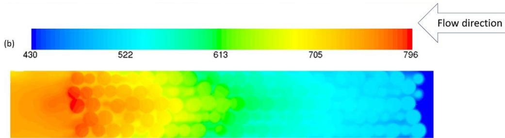
Figure 1. Contours of temperature (K) profile evolution along the tube. Inlet temperature has been decreased but temperatures in the center of the bed have increased from the steady-state values, demonstrating “wrong-way” behavior with variations at the local scale.
