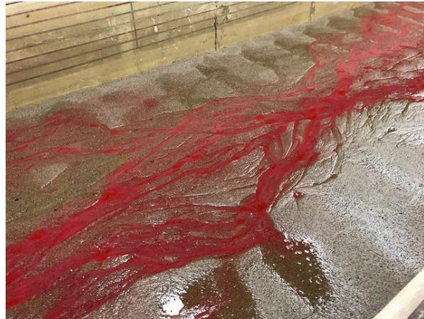
**Figure 1.** A downstream-looking view of a braided channel belt in the laboratory. Flow is dyed red and the flume width is 2.7 m.
