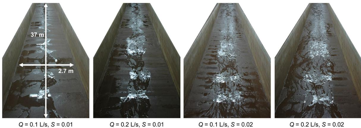
**Figure 2.** Upstream-looking views of the channel belt during each run. Water discharge ( $Q$ ) and channel slope ( $S$ ) were varied independently to test their influence on channel belt development.
