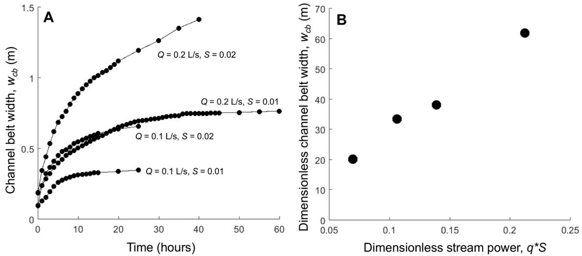
**Figure 3.** (A) Average channel belt width ( $w_{cb}$ ) versus time for each run. (B) Dimensionless channel belt width ( $w_{cb}^*$ ) versus dimensionless stream power ( $q^*S$ ), where  $w_{cb}^* = w_{cb}/L$ ,  $L = Q^{2/5}/g^{1/5}$  is a representative length scale for the channel,  $q^* = Q/(L\sqrt{gRD^3})$ ,  $g$  is gravitational acceleration,  $R = 1.65$  is the relative density of submerged sediment, and  $D = 0.42$  mm is median sediment grain size.
