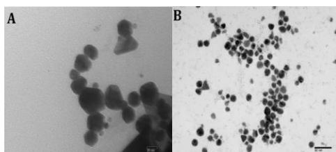
**Figure 1:** TEM images of (A.) Dex-AuNPs and (B.) Mal-AuNPs with core sizes of 20 nm and 18 nm, respectively. As TEM, imaging is the most thorough way of confirming size, shape, and dispersity of the particles these parameters for synthesis can be said to be optimum as they are the only ones, which have associated images. The Mal-AuNPs show better monodispersity in comparison to the Dex-AuNPs. However, both samples show roughly spherical particles in majority.
