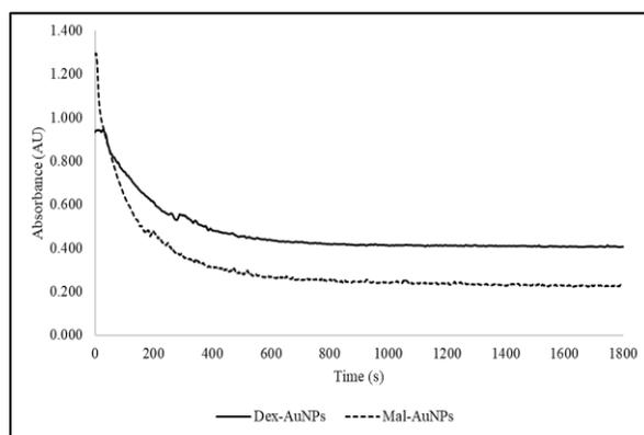
**Figure 2:** Overlay of the UV-Vis spectroscopic time scans for Dex-, and Mal-AuNPs. Each scan represents the extinction of PNP correlating to a decrease in the absorbance at 400 nm. As this reaction is carried out with  $\text{NaBH}_4$  in excess the reaction can be modeled as a pseudo-first order reaction and the rate constants for each type of AuNP determined from the respective integrated rate law.
