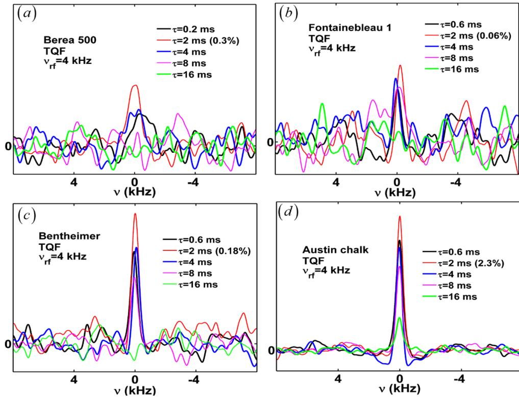
Fig. 1:  $^{23}\text{Na}$  triple-quantum filtered (TQF) spectra for different delay times  $\tau$  for Berea 500 (a), Fontainebleau 1 (b), Bentheimer (c) and Austin chalk (d).  $\tau$ : 0.6 ms – black line (in the case of (a) it is 0.2 ms); 2 ms – red line; 4 ms – blue line; 8 ms – pink line and 16 ms – green line. The relative intensity of the red peak was calibrated with respect to  $90^\circ$ -pulse excitation.
