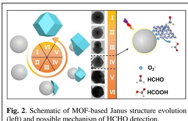
Fig. 2. Schematic of MOF-based Janus structure evolution (left) and possible mechanism of HCHO detection.
