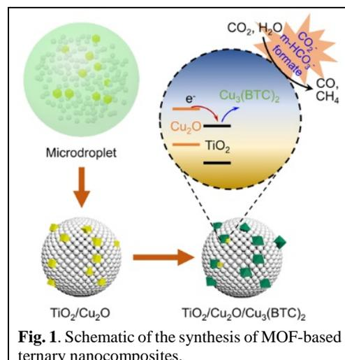
Fig. 1. Schematic of the synthesis of MOF-based ternary nanocomposites.
