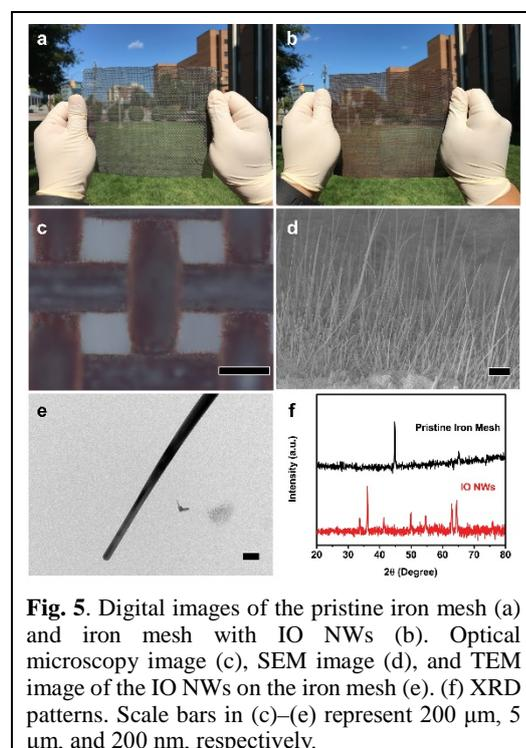
**Fig. 5.** Digital images of the pristine iron mesh (a) and iron mesh with IO NWs (b). Optical microscopy image (c), SEM image (d), and TEM image of the IO NWs on the iron mesh (e). (f) XRD patterns. Scale bars in (c)–(e) represent 200  $\mu\text{m}$ , 5  $\mu\text{m}$ , and 200 nm, respectively.
