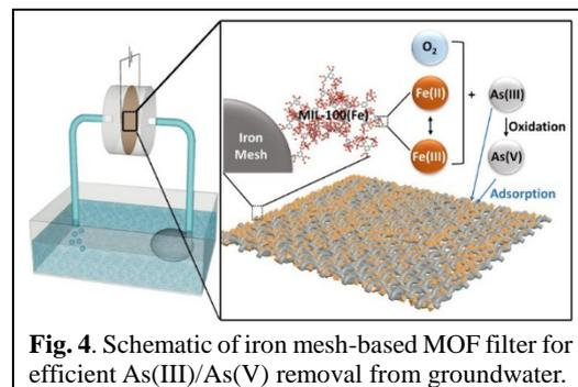
**Fig. 4.** Schematic of iron mesh-based MOF filter for efficient As(III)/As(V) removal from groundwater.
