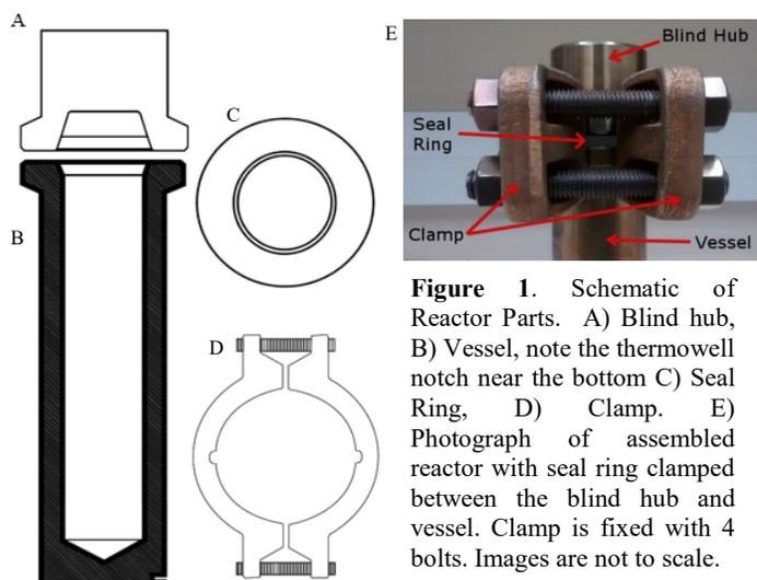
**Figure 1.** Schematic of Reactor Parts. A) Blind hub, B) Vessel, note the thermowell notch near the bottom C) Seal Ring, D) Clamp. E) Photograph of assembled reactor with seal ring clamped between the blind hub and vessel. Clamp is fixed with 4 bolts. Images are not to scale.
