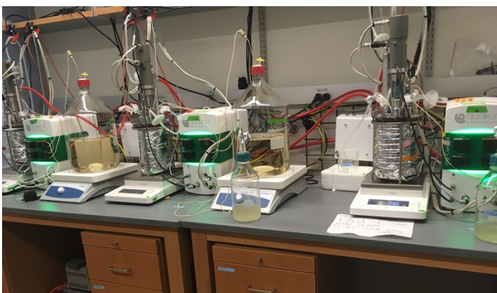
Figure 1. Leavitt lab Applikon chemostats. Operating in 3x parallel at 70°C and pH 2.5 with Sulfolobus acidocaldarius . Operated by graduate student A. Zhou.
