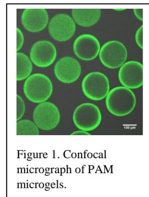
Figure 1. Confocal micrograph of PAM microgels.
