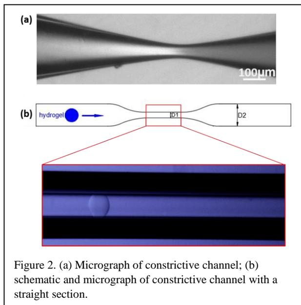
Figure 2. (a) Micrograph of constrictive channel; (b) schematic and micrograph of constrictive channel with a straight section.
