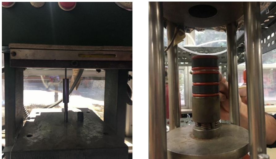
Figure 2: Experimental set up. (L) Tubular support mold in press. (R) Permeance testing reactor.
