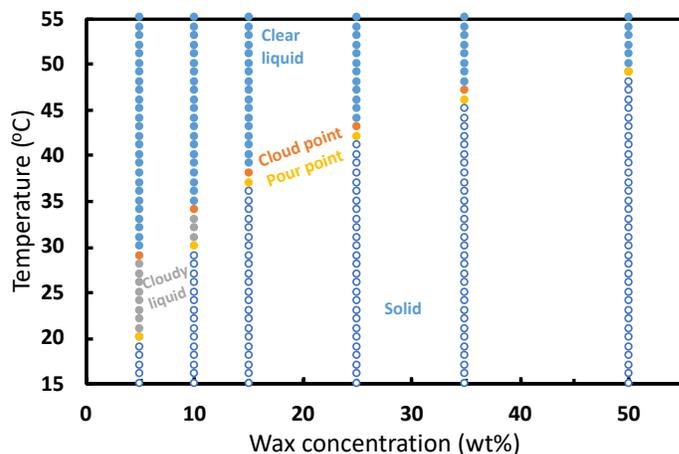
**Figure 1: Static phase diagram**
