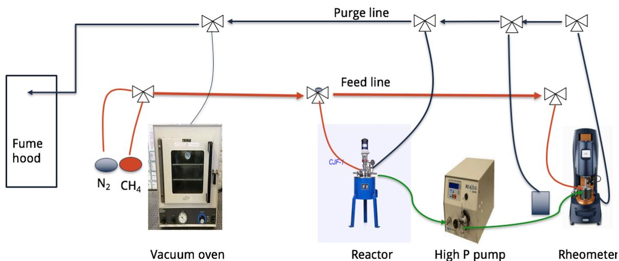
**Figure 2: Diagram of high-pressure rheology system**
