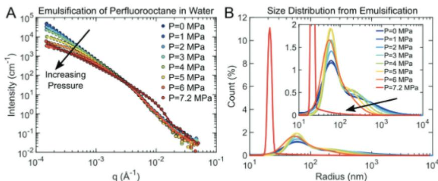
**Figure 2:** A) USAXS profiles for PFO emulsions under variable acoustic intensities. B) Droplet size distributions obtained from fits to the USAXS profiles. Cavitation only occurred when the pressure was >6.5 MPa.
