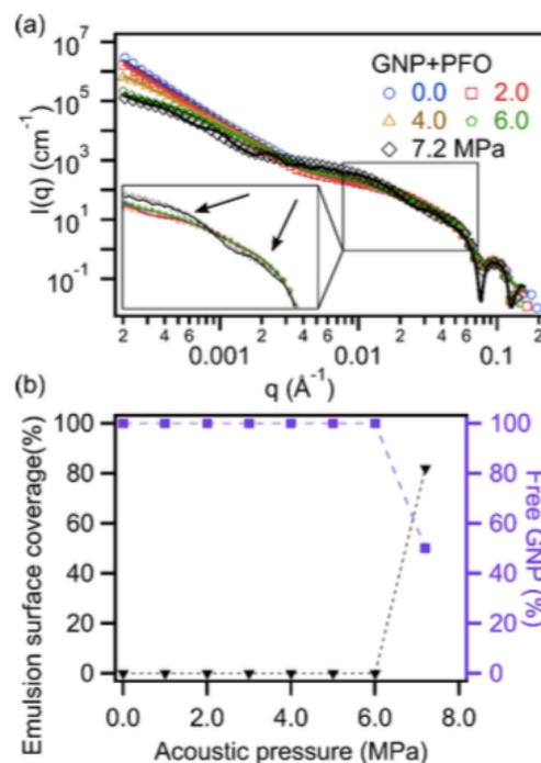
**Figure 3:** A) USAXS data and fits for PFO emulsions with gold nanoparticles (GNP) sonicated at variable pressures. B) Percent coverage of oil-water interface for emulsions and the percent of GNPs that remain ‘free’ in dispersion.
