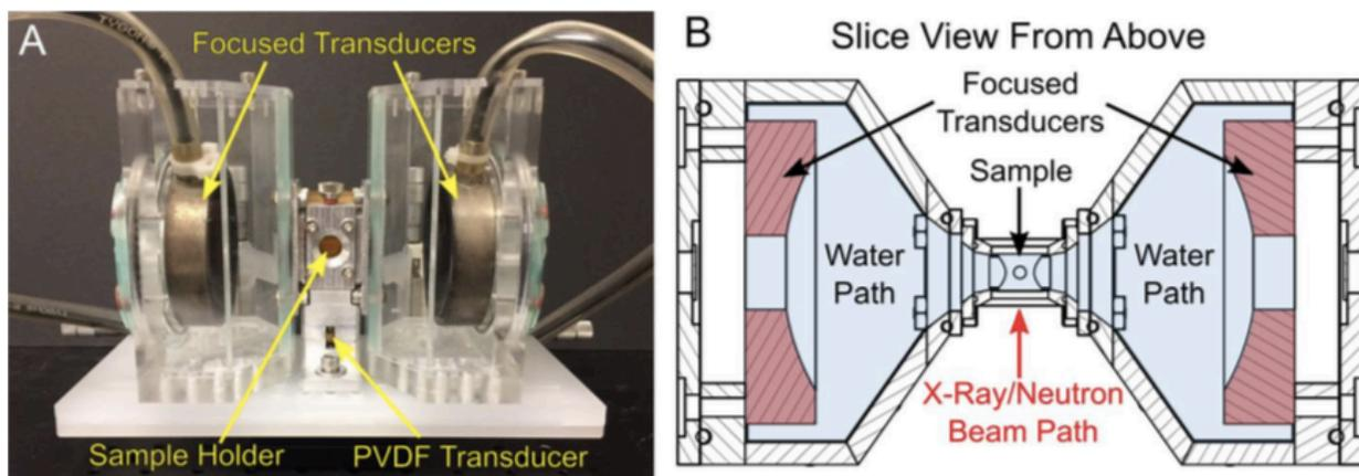
**Figure 1:** A) Photograph of the sample environment for ultrasound and SAXS/SANS analysis. B) Schematic drawing (top view) of the sample environment showing all critical components.
