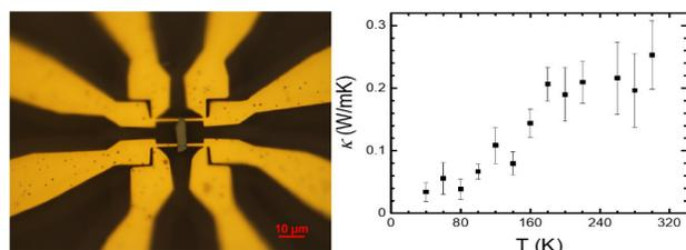
**Figure 3.** Thermal conductivity measurement of Cu-BHT. (a) An optical image of a device for the thermal conductivity measurement. The heater/sensor leads are connected to the large metal pads to measure the change in the resistance in four-terminal configuration. Cu-BHT sample is suspended between these leads. Scale bar: 10 μm. (b) Measured thermal conductivity of Cu-BHT as a function of temperature.
