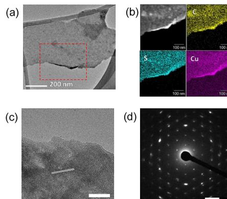
**Figure 2.** TEM images of Cu-BHT: (a) TEM image of a Cu-BHT flake. (b) STEM-DF image of Cu-BHT in the region indicated by the red dashed line box in (a), and its mapping of carbon, sulfur and copper elemental distributions using STEM-EDS. (c) HR-TEM image showing a Cu-BHT lattice with a lattice spacing of 0.76 nm. Scale bar: 20 nm. (d) Selected Area Diffraction (SAED) image highlighting the hexagonal lattice structure of the material. Scale bar: 2 nm<sup>-1</sup>.
