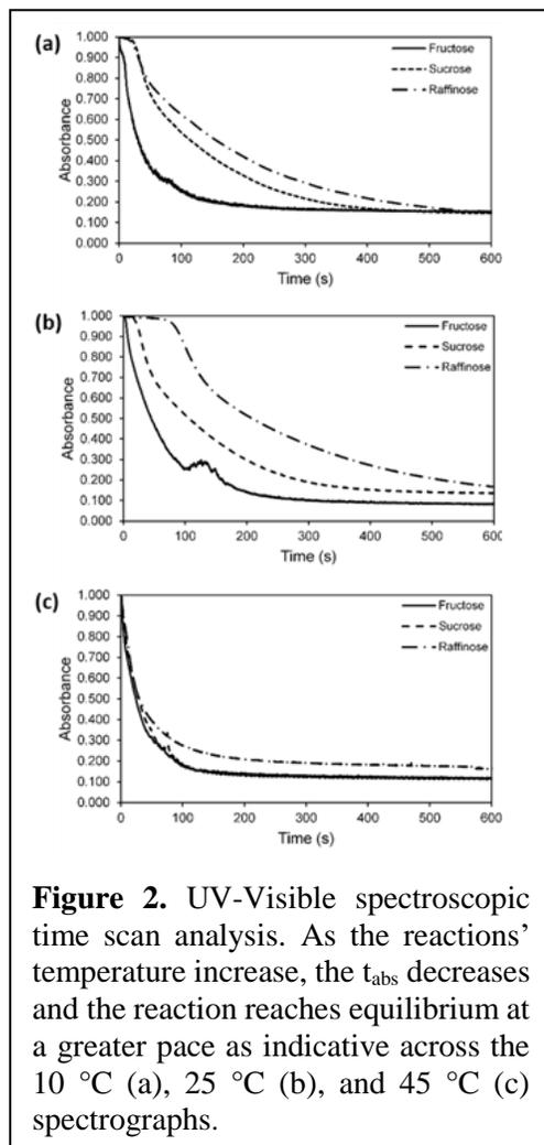
**Figure 2.** UV-Visible spectroscopic time scan analysis. As the reactions' temperature increase, the  $t_{\text{abs}}$  decreases and the reaction reaches equilibrium at a greater pace as indicative across the 10 °C (a), 25 °C (b), and 45 °C (c) spectrographs.
