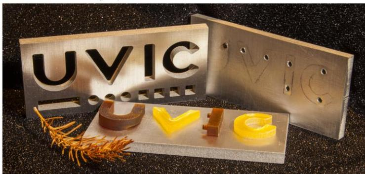
Figure 4. Macro-scale functionalized PDCPD objects produced in a reaction injection molding process.
