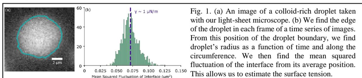
Fig. 1. (a) An image of a colloid-rich droplet taken with our light-sheet microscope. (b) We find the edge of the droplet in each frame of a time series of images. From this position of the droplet boundary, we find droplet's radius as a function of time and along the circumference. We then find the mean squared fluctuation of the interface from its average position. This allows us to estimate the surface tension.
