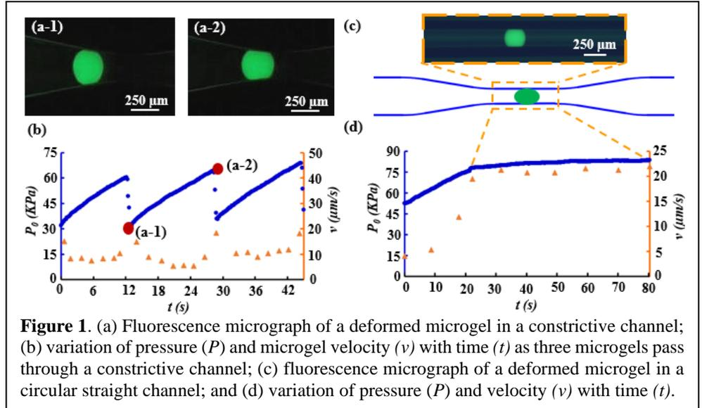
**Figure 1.** (a) Fluorescence micrograph of a deformed microgel in a constrictive channel; (b) variation of pressure ( $P$ ) and microgel velocity ( $v$ ) with time ( $t$ ) as three microgels pass through a constrictive channel; (c) fluorescence micrograph of a deformed microgel in a circular straight channel; and (d) variation of pressure ( $P$ ) and velocity ( $v$ ) with time ( $t$ ).
