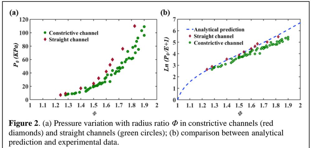
**Figure 2.** (a) Pressure variation with radius ratio  $\Phi$  in constrictive channels (red diamonds) and straight channels (green circles); (b) comparison between analytical prediction and experimental data.
