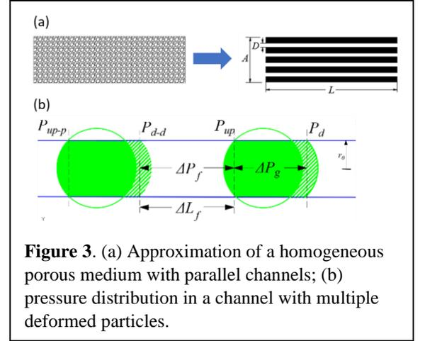
**Figure 3.** (a) Approximation of a homogeneous porous medium with parallel channels; (b) pressure distribution in a channel with multiple deformed particles.
